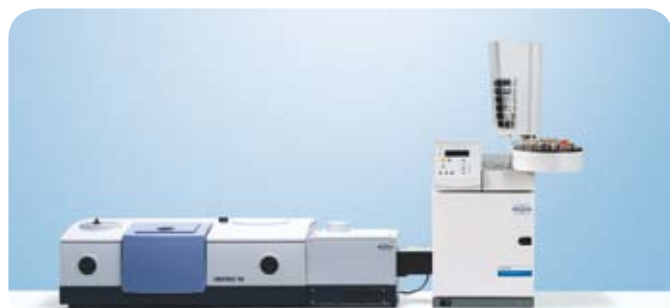
Picture 1 GC-IR accessory placed in between the GC and the FT-IR
