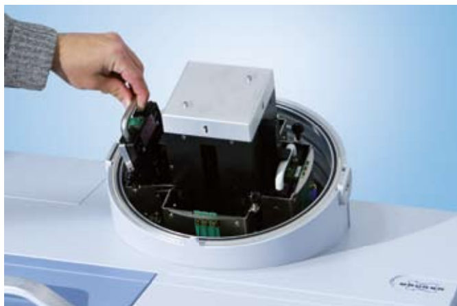
Fig. 2: The open cover shows the inserted four beamsplitters mounted in the BMS-slots of the exchange unit BMS-c
